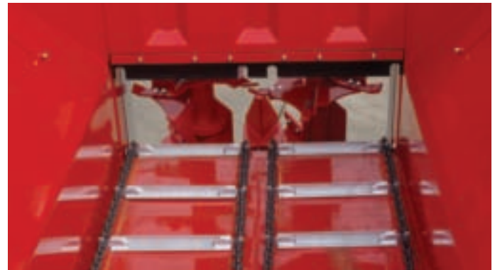
4 floor chains for strength and durability
