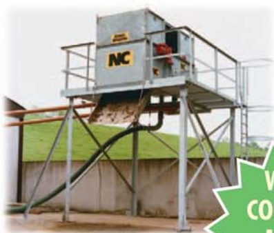
The fibre slides down a stainless steel chute ready to stack for composting
